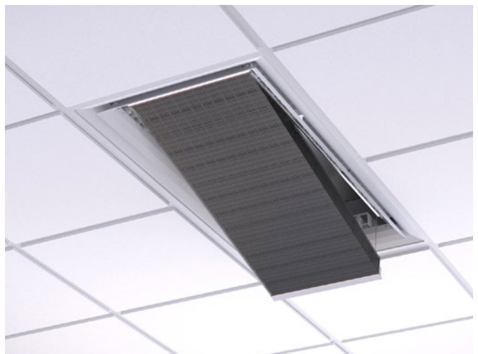
Figure 15. Removing the face plate and folding out the coil for accurate cleaning in the event of high hygiene requirements. Note! requires the product to be ordered with the accessory, fold-out coil, and that flexible connection hoses are used on the water side.
