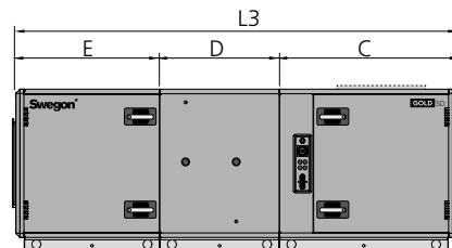
Fan + filter + coil heat exchanger
