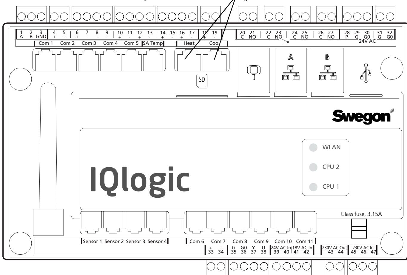
Digital inputs, terminals 4-17, are of extra-low voltage type. Analogue input, terminals 18-19 have an input impedance of 66 kΩ. 230 VAC control voltage is on external terminals 101 (L) and 102 (N).
