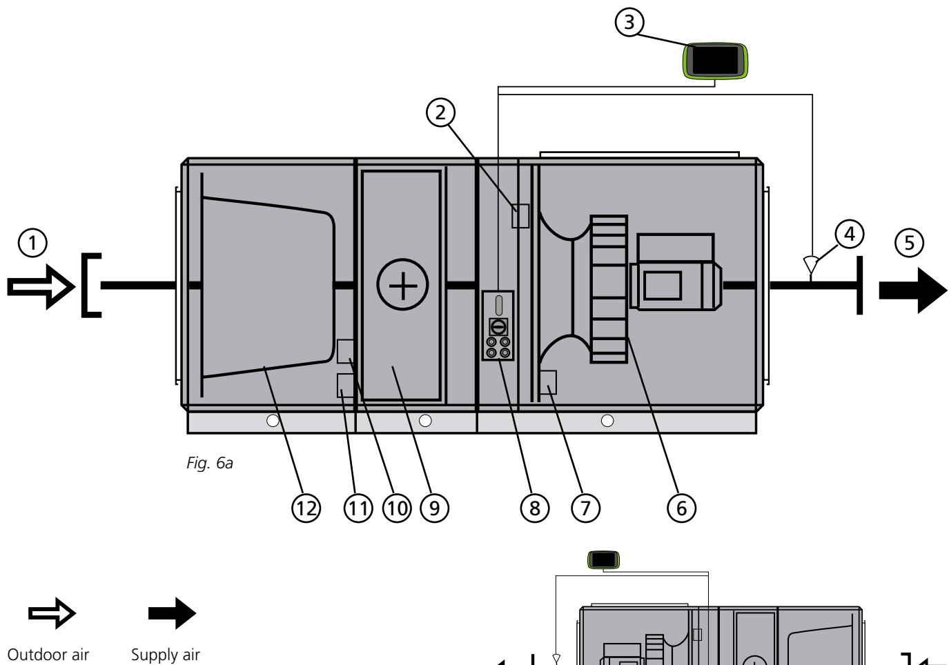
The air handling units can be ordered in the right-hand version as shown in Fig. 6a or the left-hand version as shown in Fig. 6b. The air handling units can also consist of filter and fan only or fan only.
