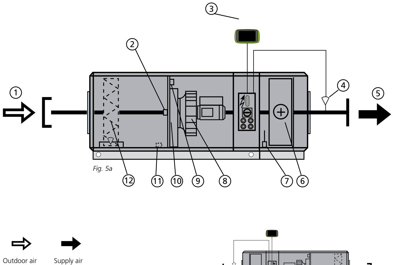
The air handling units can be ordered in the right-hand version as shown in Fig. 5a or the left-hand version as shown in Fig. 5b. The air handling units can also consist of filter and fan only or fan only.
