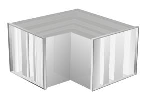
Figure 1. The LENTO produces a uniform velocity distribution downstream of the bend by utilizing the acoustic baffles as guide vanes.
