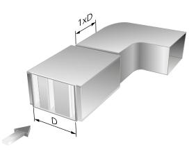
Figure 5. Sound attenuator upstream or downstream of a bend
