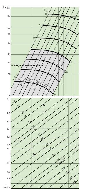
**Diagram 1. Correction for different connection**
