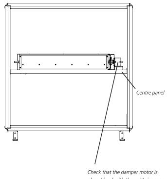
check that the damper motor is placed level with the unit's inspection doors.
