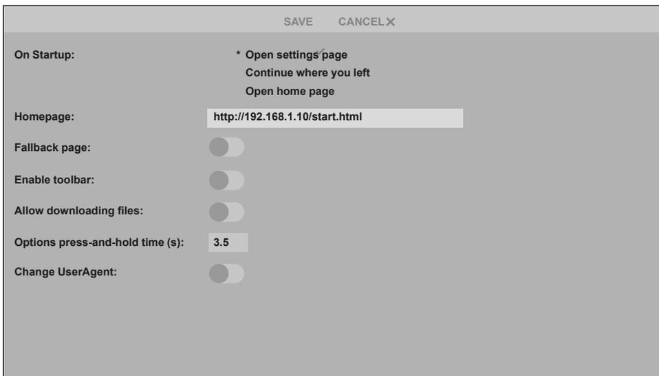
2. Change the preset address: `http://192.168.1.10/start.html` to the same IP address as in the PLC system and press "SAVE".
