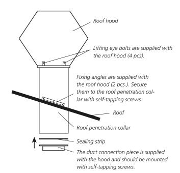
The hoods for the size 04-12 GOLD/SILVER C and size 02-03 COMPACT units have circular duct connection fitted with a type-approved rubber ring seal for jointing to spiral ductwork. The hoods for the size 14-40 GOLD/SILVER C units have rectangular duct connection for slip-clamp joint connection.
