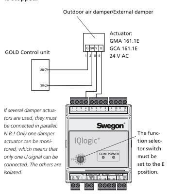
Under normal operating conditions, the damper opens and closes by means of the damper actuator's motor drive (actuating time: 90 seconds).
