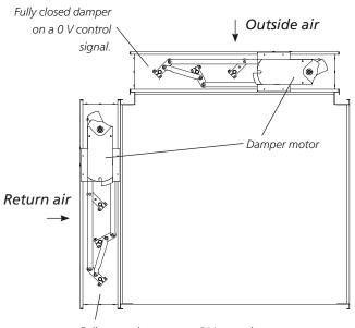
Fully open damper on a 0 V control signal. The direction of travel of the damper actuator must be changed. See Item 6.
