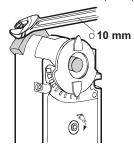
Remove the damper actuator from the damper spindle. It might be necessary to also remove the lower bracket.
