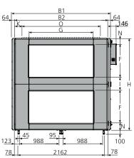
\* The air handling unit is supplied without end connection panel if a duct accessory housed in an insulated casing will be connected. The AHU can also be supplied with full face end connection panel (accessory).
