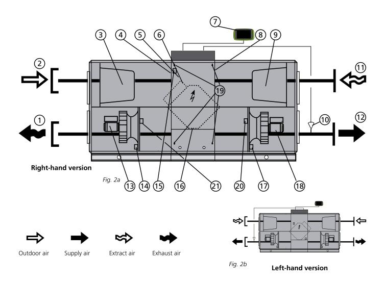
The air handling units are supplied in the right-hand or left-hand version as shown in Fig. 2a and 2b. In the left-hand version (Fig. 2b), the components marked with an asterisk change function and designation (the components are named according to whether the function is for supply air or extract air.).
